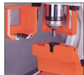
Goose-neck die holder for punching channel flanges and web
