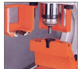
Goose-neck die holder for punching channel flanges and web
