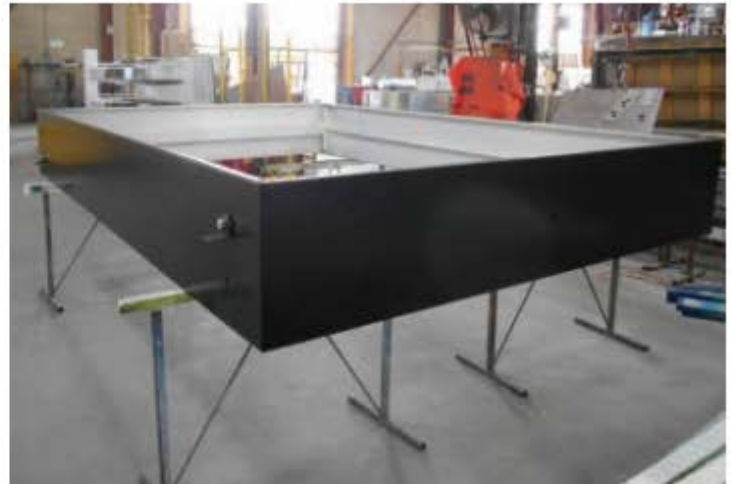
This is an example of a filler, which is formed to make the box that holds LED lighting and power supplies to light up a sign.
