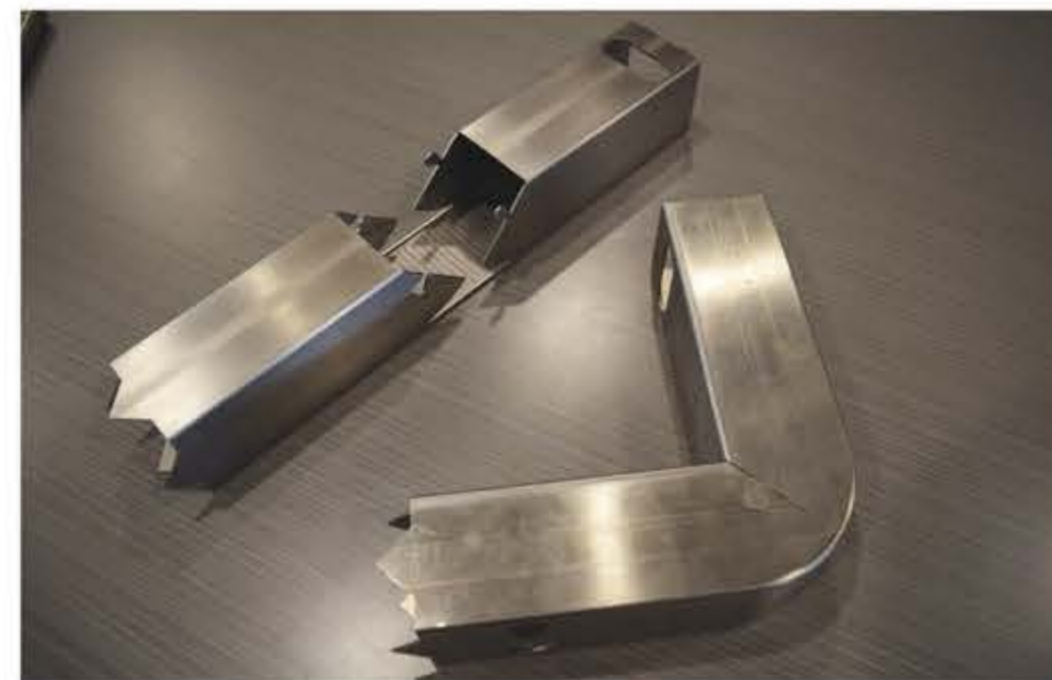
One of the values of a tube laser is how it can simplify welding setups and assemblies. Here we see a part that has been tube cut and assembled with a slot and tab arrangement to simplify weld setup and a shallow series of cuts to aid in bending.
