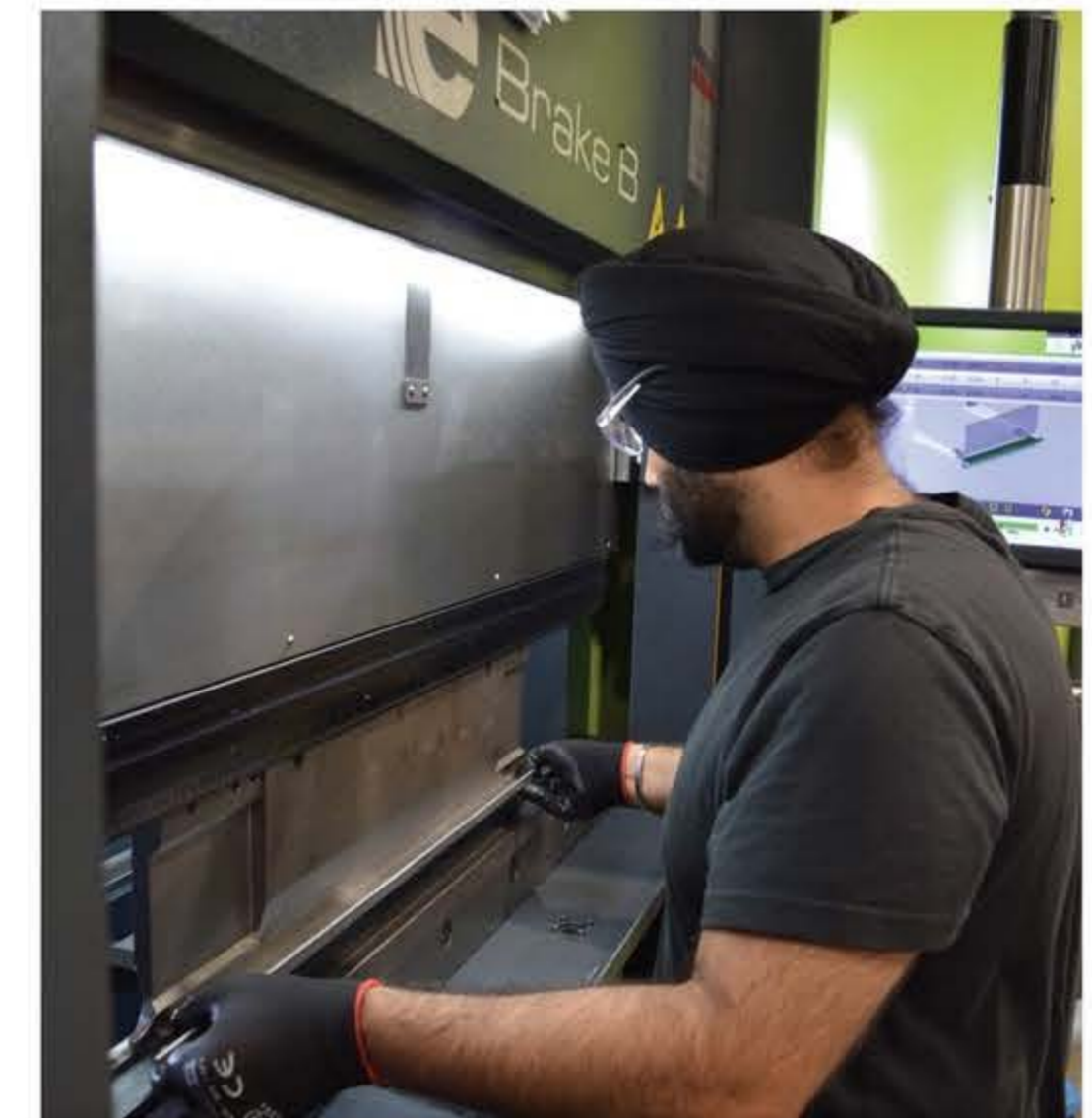
The smaller, 40-ton SafanDarley model is suitable for quick turnaround of smaller parts. Millomat owner Mani Sehmbi said, "When we did tests, we found that with the electric brake we were doing parts in half the time that a hybrid could produce them."
